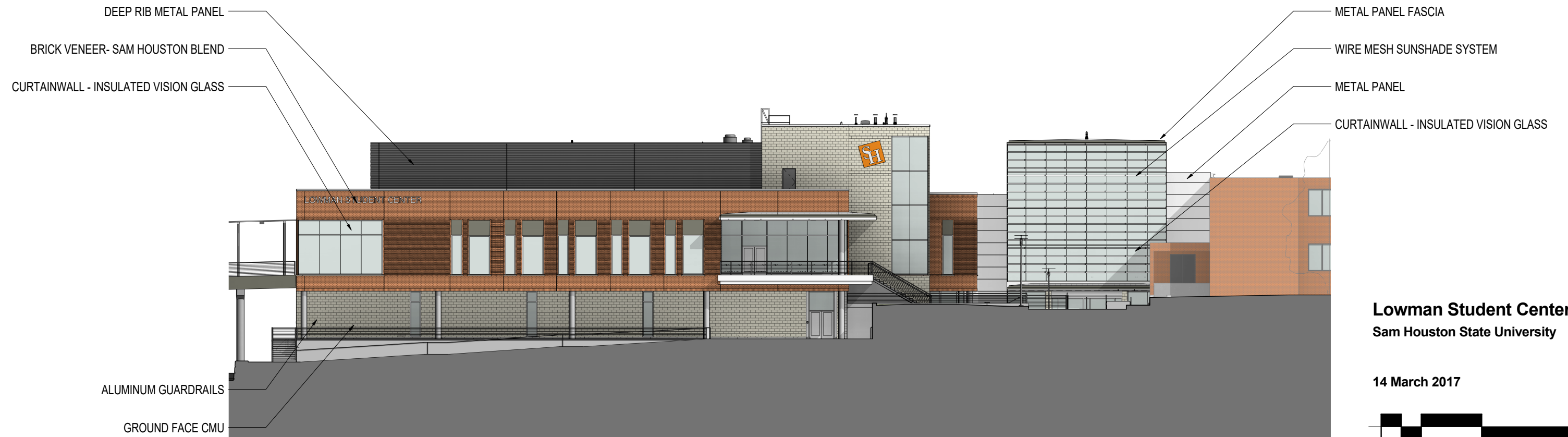
WEST BUILDING ELEVATION
