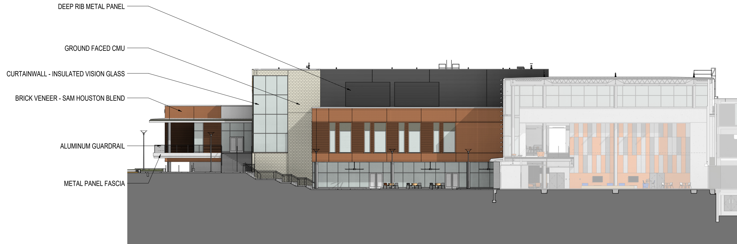
SOUTH BUILDING ELEVATION
